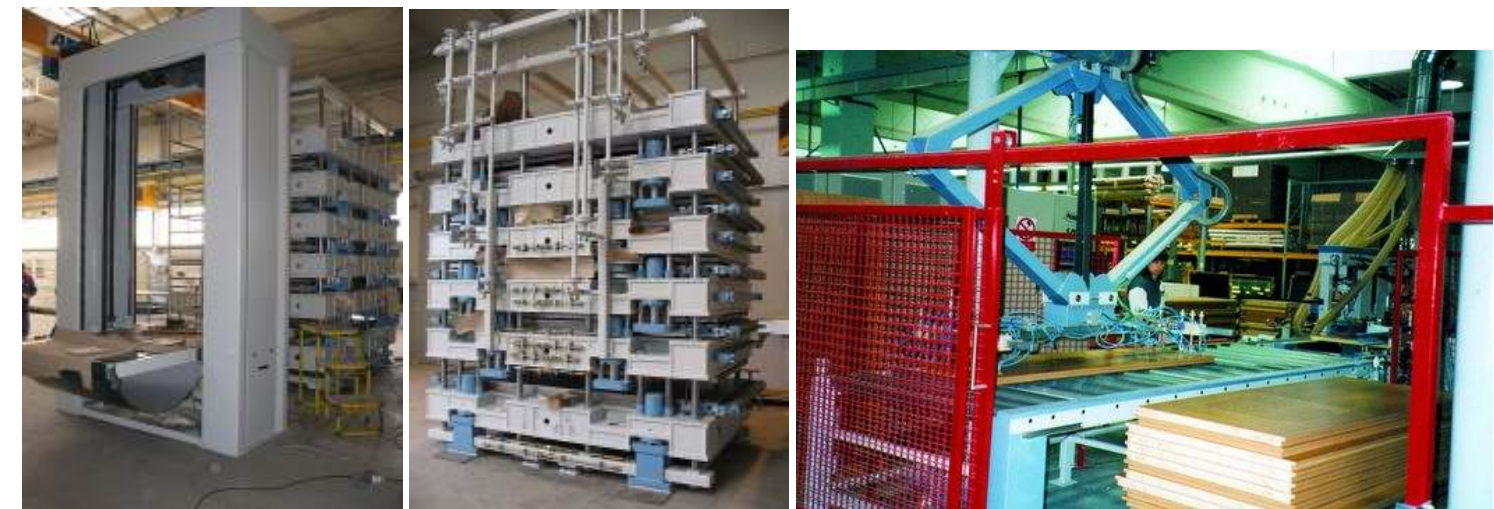
Press lines for door production
