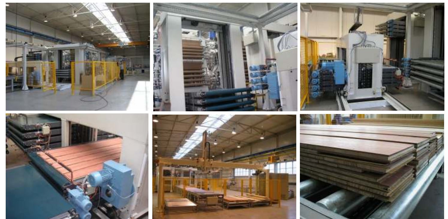
Press lines producing wooden parquets
