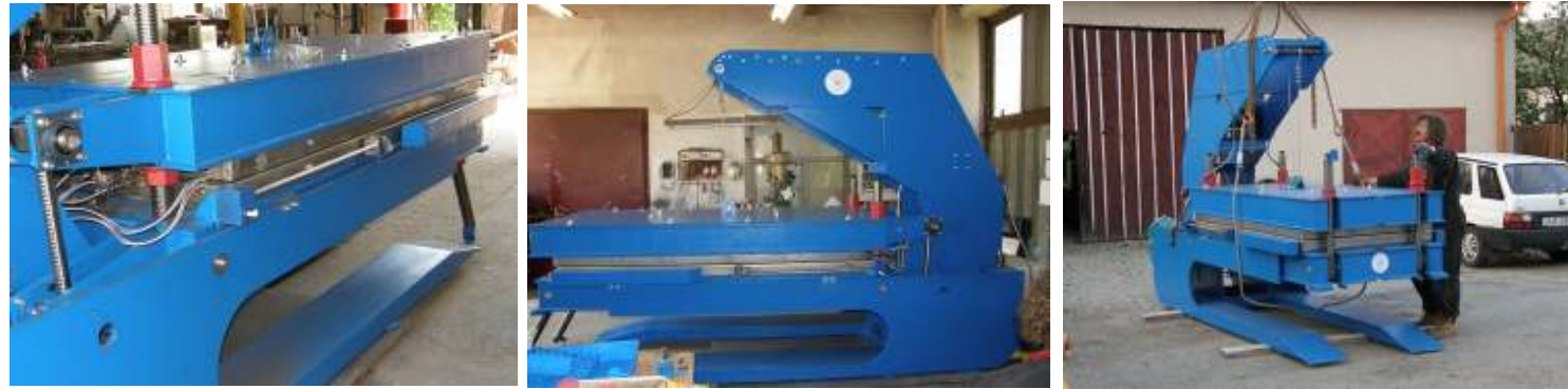
Presses for rubber conveyor belts joining by vulcanization
