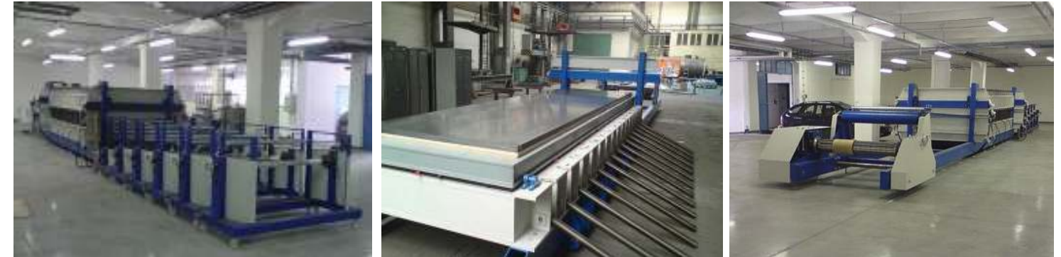
Press lines for rubber and syntetic conveyer belts production ( belts ase used for transport of coal, sand, grain or corn ).
