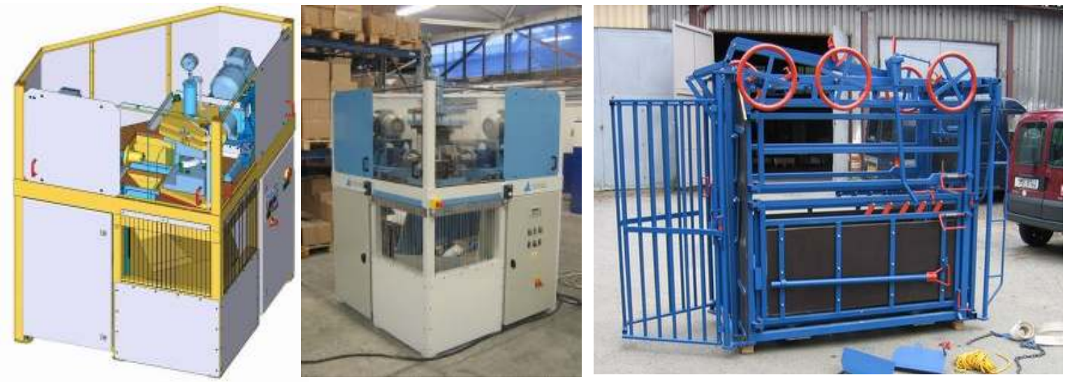
CAD -3D design → product Machine for stainless-steel elbow forhead machining
